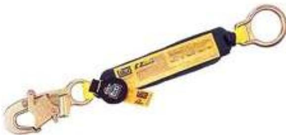
A 100kg person who is jerked to a stop after falling 2 metres generates a force on a lanyard without a shock absorber approximately equivalent to a 1500kg mass. If there is no shock absorber this will either cause a severe injury or cause the lanyard or harness to fail resulting in severe injury.
