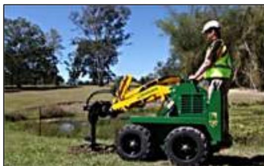
Mini-loaders can be difficult to operate on wet, slippery slopes and uneven ground.
