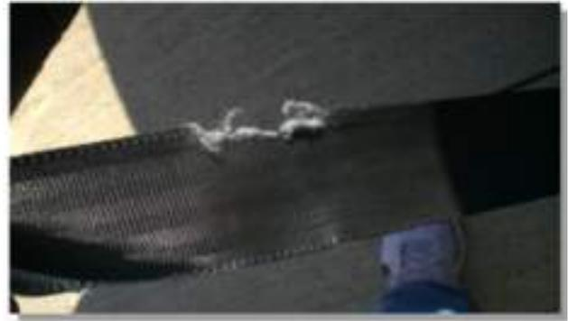
*Fraying seatbelts should be replaced.*
