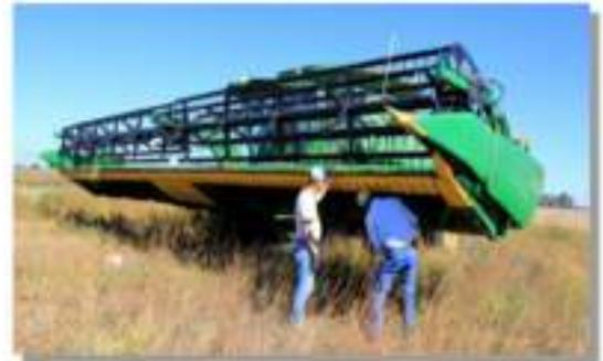
*The header of a combine should be adjusted to suit the crop and the weather conditions.*
