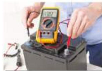
*A voltmeter enables you to check the charge in a battery. Source: yourmechanic.com*
